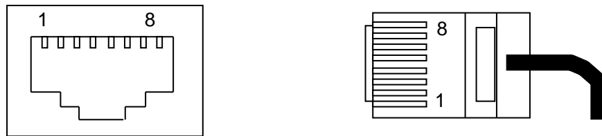
7: Receive data 8 : Transmit data 6 : Ground
