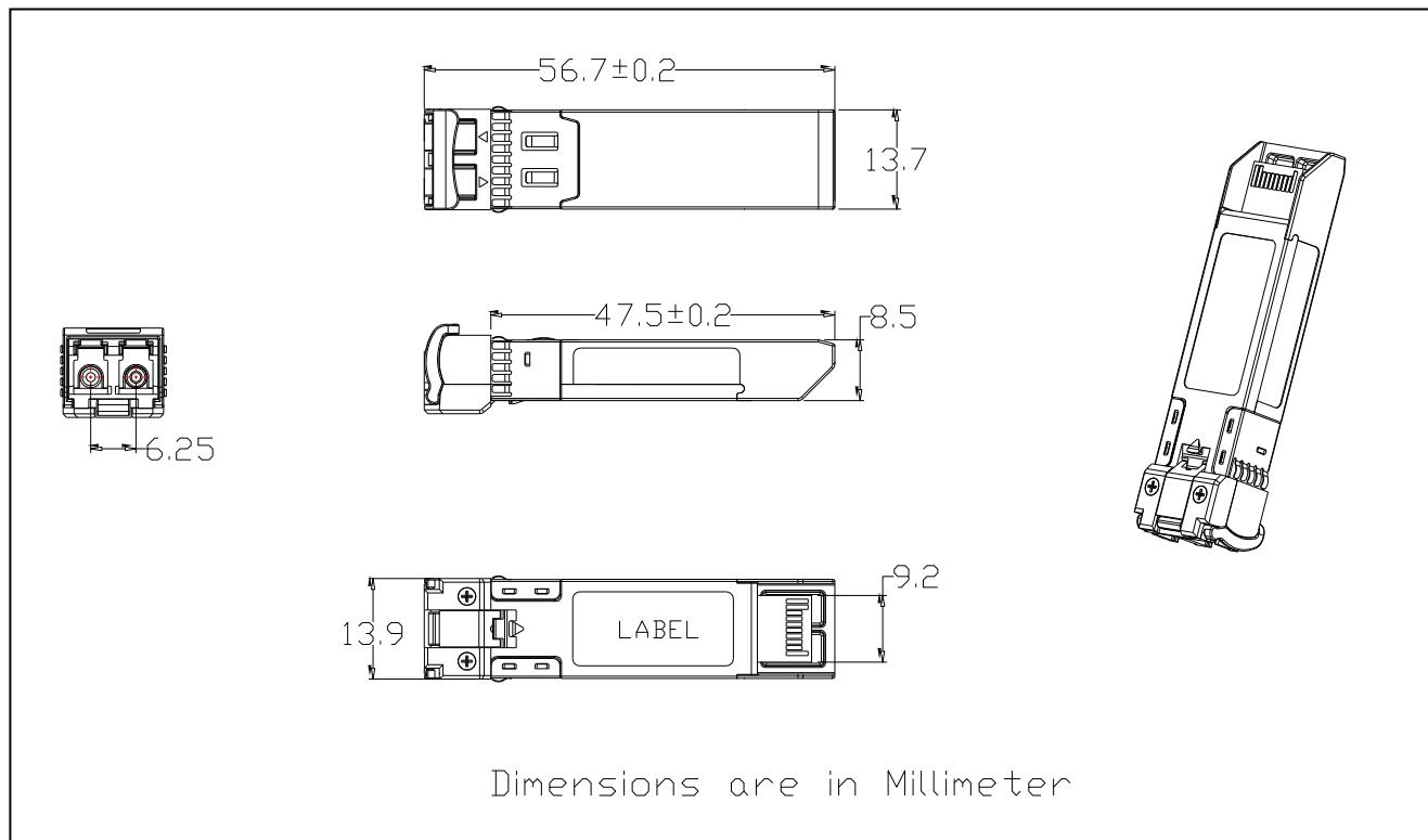
Tolerance without indication is  $\pm 0.1\text{mm}$
